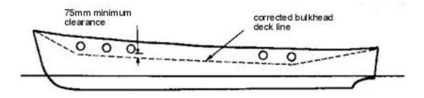
Figure A3-5: Raised deck vessel
