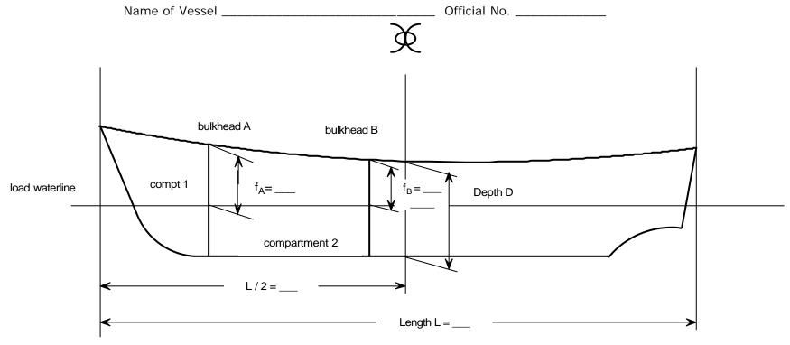
Figure A3-1 – Profile of vessel
